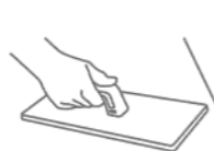
COMPRESSING THE TILE
